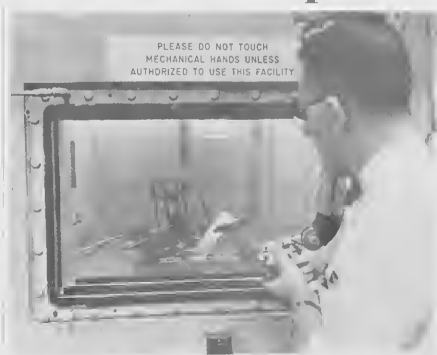
SCIENTIST manipulates mechanical hand grasping radioactive material. SCIENTIFICO ta manipulá mannan cu ta cage material radioactivo.
